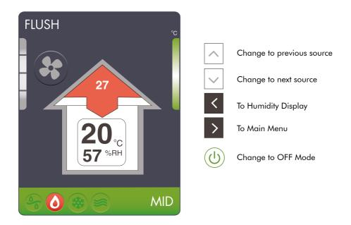
FLUSH will cause the fan to work at full speed for up to two hours. Great for flushing out odours or if there is excess moisture in the home (burnt toast, cooking smells, steam cleaning, etc).
