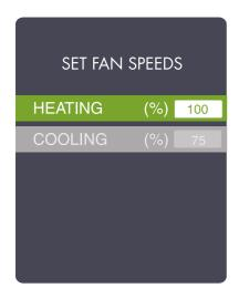
The Fan Speed Menu is used to set the maximum available fan speeds in the Heating and Cooling Modes.
