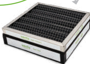
Premium Ventis filter Carbo & Nano filtration to 0.3 micron MERV13
